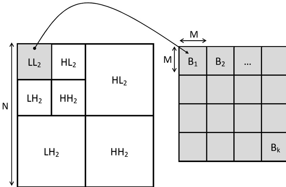
Figure 2.  $LL_2$  sub-band is divided into sub-block
