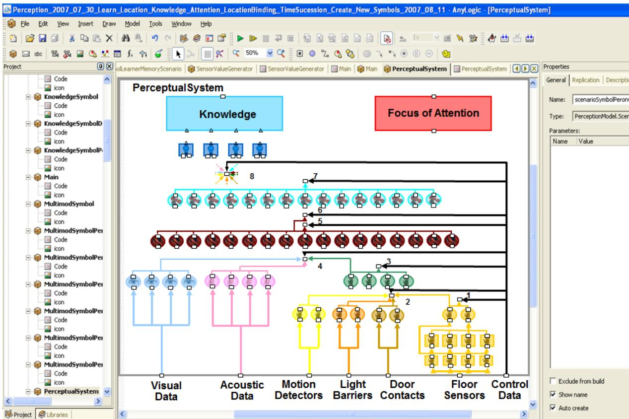
Figure 14. Implementation of Overall Architecture of the Perception Model in AnyLogic
