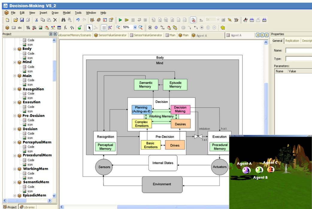
Figure 19. AnyLogic Implementation of Decision-Making Architecture in a Virtual Autonomous Agent Environment
