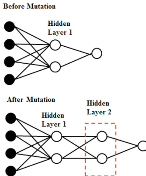
Figure 5. Insertion and Deletion Hidden Layer in NN
