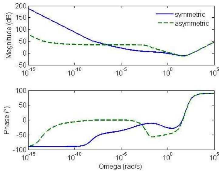
Figure 2: Impedance by means of Bode-plot representation, symmetric (continuous line) and the asymmetric (dashed line) tree.
