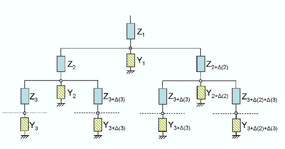
Figure 1: Asymmetric representation for the first four generations, in its electrical equivalent
