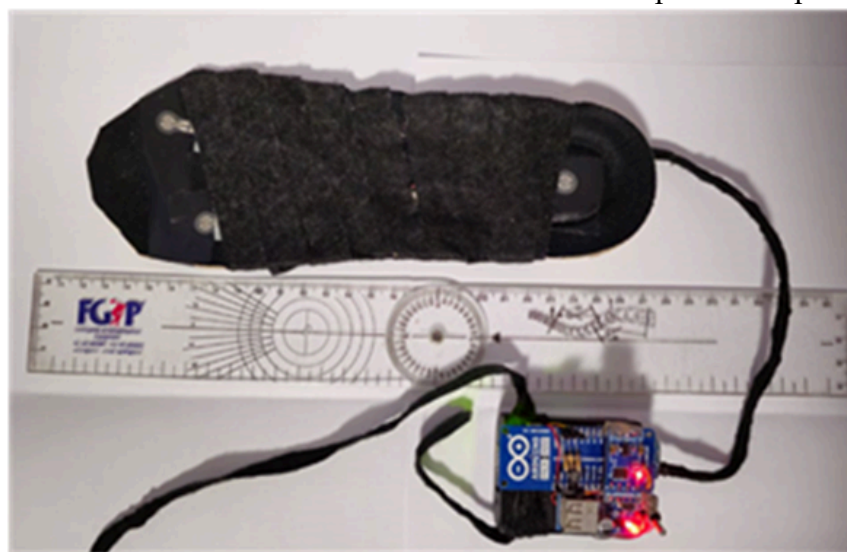
Figure 5. Real-time biofeedback device (Arduino MKR1000 + ADXL345 + three FSRs). Function: immediate, rule-based visual feedback for gait re-education (no AI).
