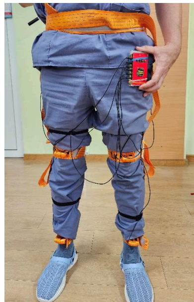
Figure 7. The STM32 wearable system with six synchronised accelerometers during tests
