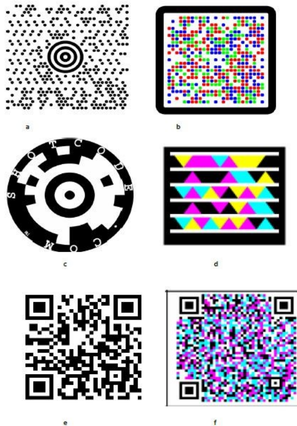
Figure 4. 2D barcode examples a) MaxiCode b) CrontoSign c)ShotCode d)HCCB e)QRcode f)HCCBQ
