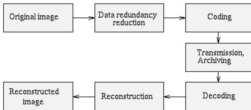
Figure 3. Data compression and image reconstruction (55:148 Digital Image Processing, 2017)
