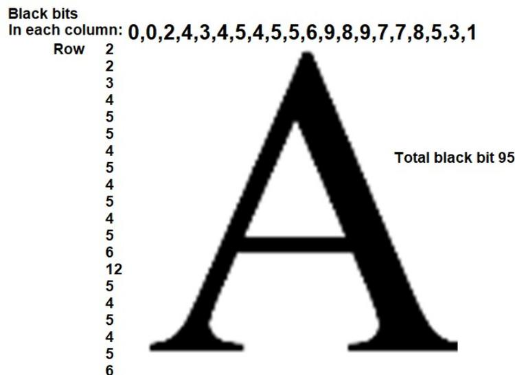
Figure 8. Sample Data Extraction for a 20\*20 size image
