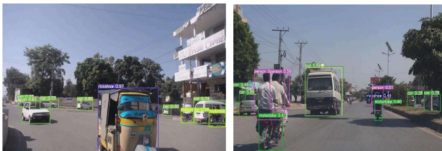
Figure 11. Object detection results of the single-stage detector on the proposed data collection
