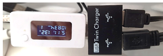
Figure 8. An example of the USB multimeter KCX-017 usage in the experiment
