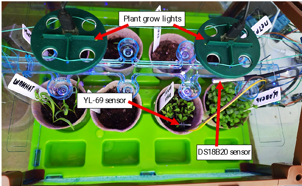
Figure 5. Installation of the DS18B20 temperature sensor, YL-69 soil moisture sensor, and two LED grow lights inside a smart \mu GH
