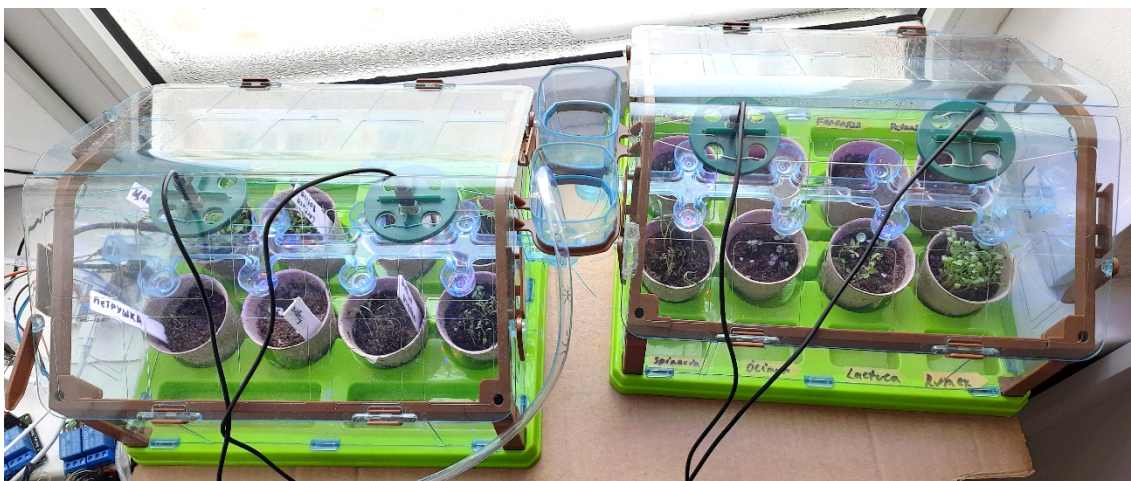
Figure 2. Commercially produced \mu GHs used in the study (with IoT smart equipment on the left and without it on the right)
