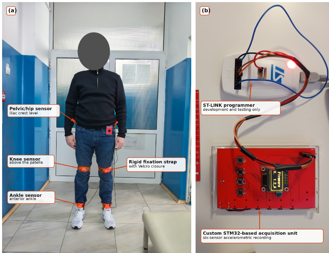
Figure 1. GaitFlow Scanner wearable accelerometry system. (a) Six-sensor configuration used during system development and testing, with accelerometers positioned bilaterally at the hip, knee, and ankle levels and secured with rigid fixation straps with hook-and-loop (Velcro) closures. The person shown is the author and not a study participant. (b) STM32-based acquisition unit used to record synchronised data from six triaxial accelerometers.
