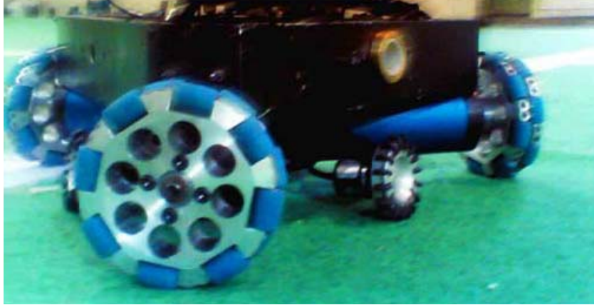
Figure 2 Three omni directional wheels act as actuators while three free wheels are for feedback.
