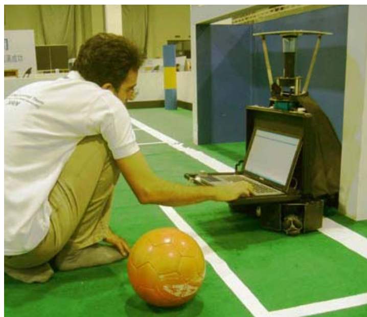
Figure 1 Our robot is a 3-wheeled omni-directional mobile robot with an omnidirectional vision system, a normal camera and a kicking device, and is controlled by a notebook PC. The chassis of the robot is designed as a frame construction where there is the electronic circuit board, batteries, kicking device, motor controller and notebook PC. The omnidirectional vision system and the normal camera are on the top of the framework.
